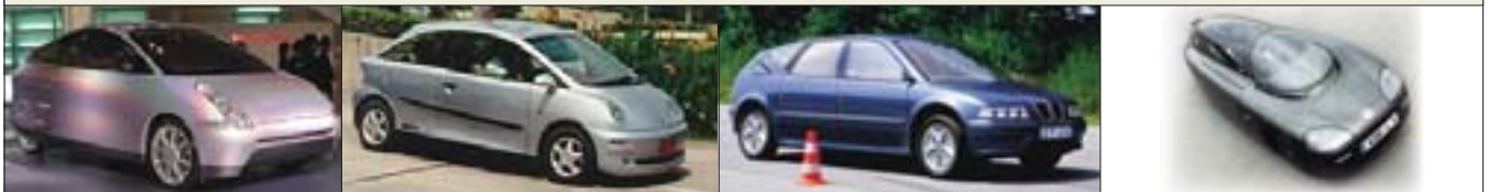
Figure 13: Four composite concept cars: From L–R, they are: Daihatsu 2003 2+(2)-seat UFE-II hybrid (569 kg, carbon-fiber, C_d 0.19, 141 mpg on Japanese 10/15 cycle, by-wire); 282 1996 4-seat Coupé (1,080 kg including 320 kg/25 kWh NaNiCl batteries, pure-electric, 100-mi range with a/c on, 12–20 DC kWh/100 km, 114–190 mpg-equivalent) developed by Horlacher in Switzerland for Pantila in Thailand; BMW 1999 Z22 (~20 body parts, ~1,100 kg [~30% weight cut] via carbon and other composites and light metals, 39 mpg, by-wire); 283 VW 2001 "Ein-Liter-Auto" 2-seat tandem 1-cylinder diesel 284 (carbon fiber, 290 kg, C_d 0.159, 8.5 hp, 74 mph, 238 mpg). 285 (A 1990 carbon/aramid 2-seat Swiss electric car weighed just 230 kg without batteries.) 286
